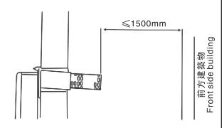
廢氣回流可能導致不正常燃燒而引致火警。 Abnormal combustion may take place by returned exhaust air to cause fire.
