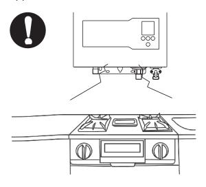
煮食爐具的廢氣及油膩物質可能損壞熱水爐。 The heater may be damaged by exhaust air and oily materials produced by cooking appliances
