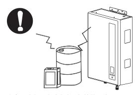
氯氣混合物對人體有害及損壞熱水爐。 A corrosive gas produced by chlorine compound is harmful to human body and the heater may also be damaged. ■確定熱水爐已接地。
