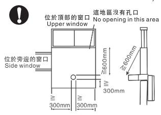
若廢氣回氣入室内,可能導致産生有毒一氧化炭。 If the exhaust air returns inside the room,a carbon monoxide toxication may be caused.
