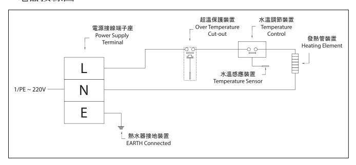
The heater must be connected to a professionally installed (as fig. above) with earthed outlet and compliance with domestic E lectrical Products (Safety) Regulation. Multiple connectors must not be used.
